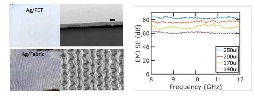
The team is coating Electroninks' reactive silver inks a variety of flexible substrates such as PET and fabric for high performance EMI shielding
