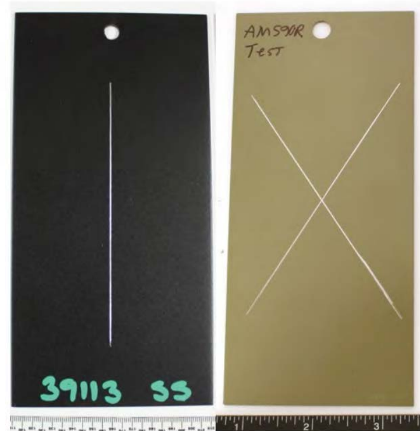
Fig. 2 Examples of a single linear scribe (left) and an X-scribe (right).
