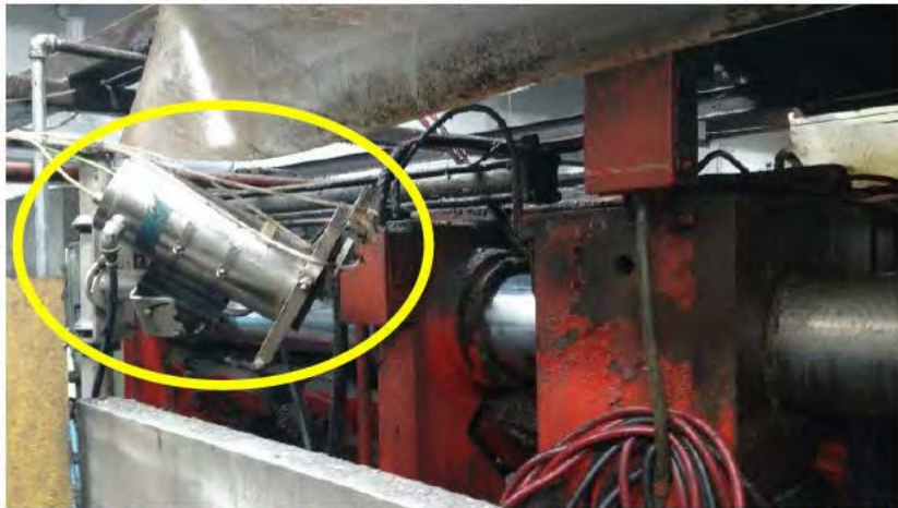
Figure 3 – Thermal Image Camera System Installed on Die Cast Machine
