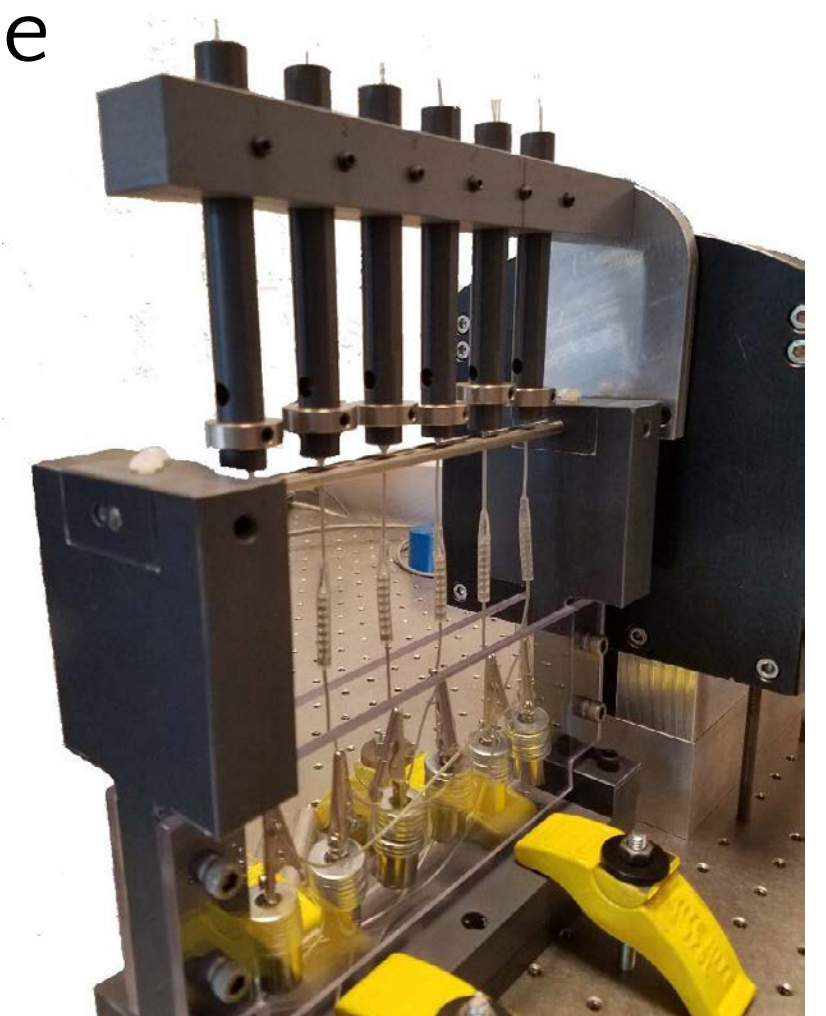
Multi-specimen flex bending fatigue
