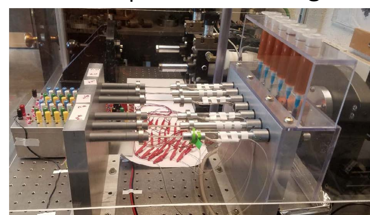
Multi-specimen rotational fatigue showing functional monitoring
